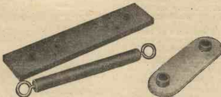
Three home-made insulators. That on the left is an ebonite strip drilled to take aerial and rope, while ebonite inserts are used in the right-hand one.
