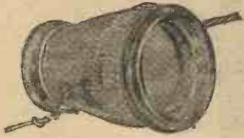
A small jar makes a very efficient insulator.
