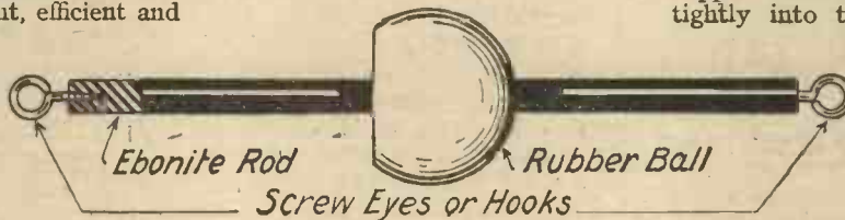
Fig. 2.—A "low-loss" insulator of novel construction. If a stout ball is used there will be no tendency for the rubber to sag.
